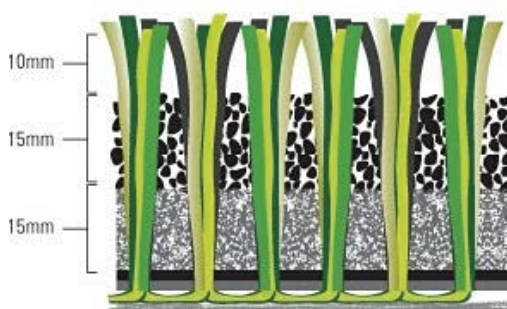
Figure 1. An artificial grass system consists of fibres (grass threads), backing (substrate to which the fibres are attached), sometimes wrapping wires (wires that attach the fibres to the substrate), often a shock pad and granules. Illustration from Alphaturf.
