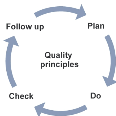
Figure 1-2. Structure of the quality system.
