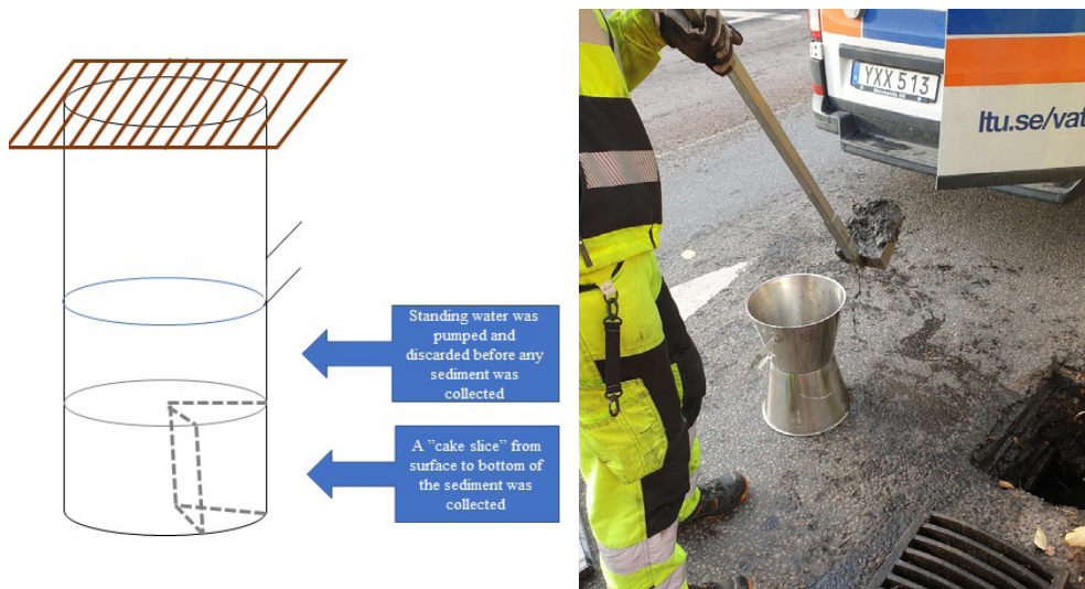
Figure 5. A schematic description of how the sampling of gully pot sediment was conducted (left) and the tool used for retrieving the sediment from the gully pots (right).
