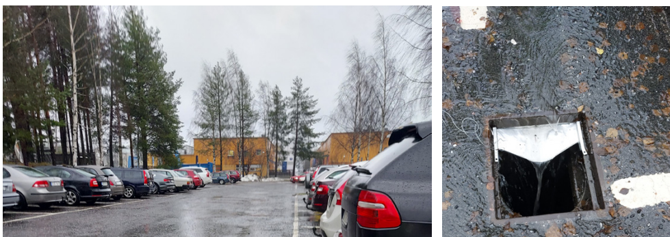
Figure 2. The PL parking lot catchment (left) and the arrangement with a funnel/spout at the gully pot inlet to facilitate the sampling (right).
