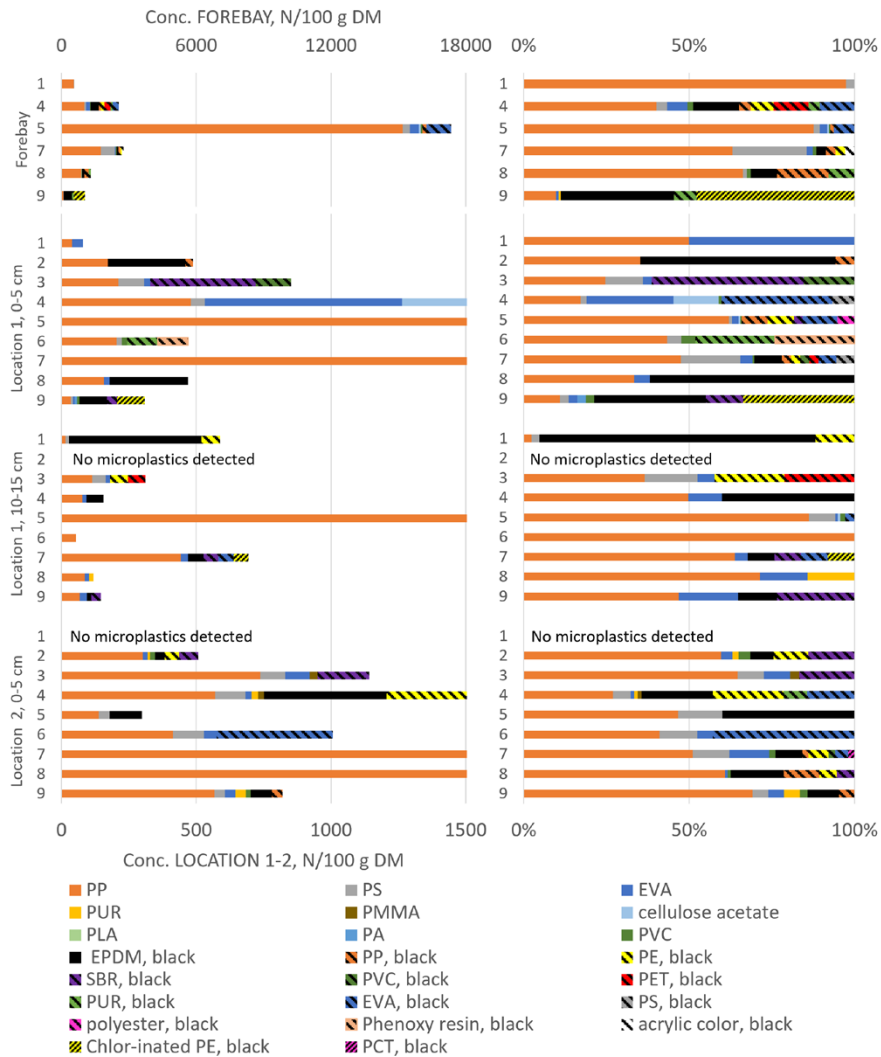
Figure 11 Microplastic concentration (left) and composition (right) of filter media from different locations (forebay, location 1, and location 2) and depths (0-5 cm and 10-15 cm) (c.f. Figure 7) of nine bioretention systems. Black particles were included in the analysis and are reported separately. (Graphs made from data in Table 2 in Lange et al 2023). Note that the concentrations in the forebays are presented using a different scale.
