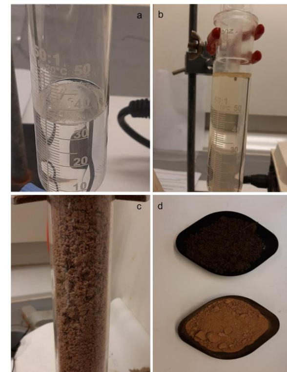
Figure 2: a) Condensate during dry out; b) Condensate at the end of the heat treatment; c) Treated soil sample; d) Comparison of untreated and treated samples: top (untreated) bottom (treated)
