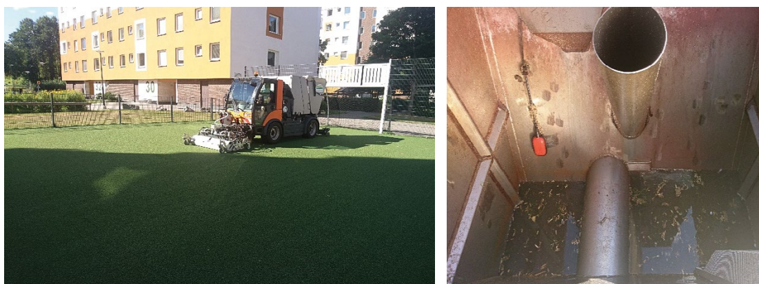
Figure 5. Sandmaster's internally produced machine for wet cleaning of artificial grass pitches with or without granulate and the collected washing water analysed by IVL.
