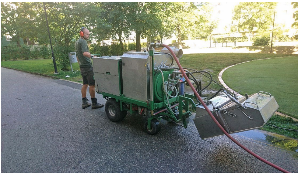
Figure 2. Sandmaster's internally produced machine for wet cleaning of rubber surfaces, which was used in the project.
