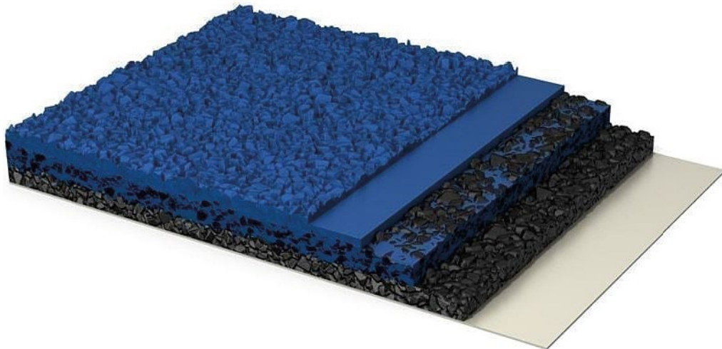
Figure 11. Design of rubber substrate for running tracks. The top layer is usually made of coloured polyurethane (PUR) or EPDM and the bottom layer of black SBR (recycled tyres). This photo shows a common running track material with the product name Tartan Gold.
