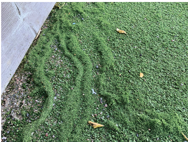
Figure 18. Extensive fibre shedding from artificial grass surface K4.
