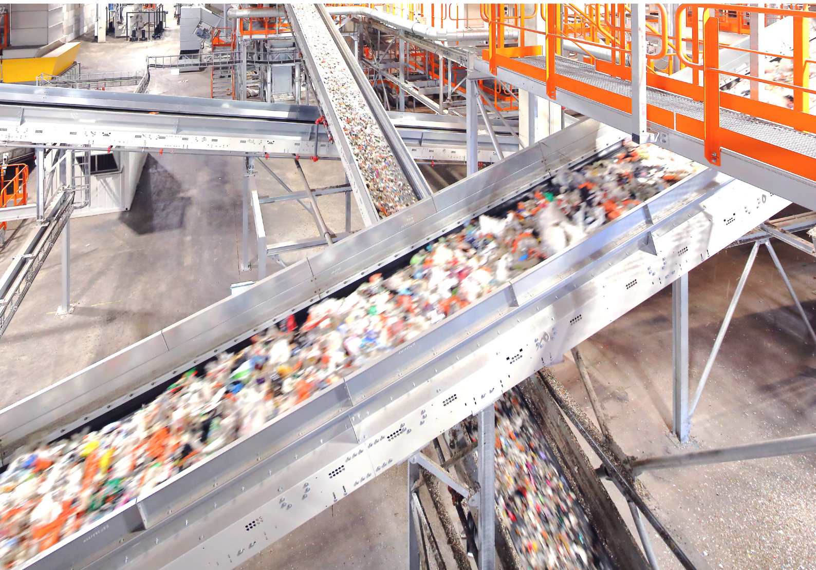
Svensk Plaståtervinning's plant in Motala sorts packaging based on the type of plastic.
