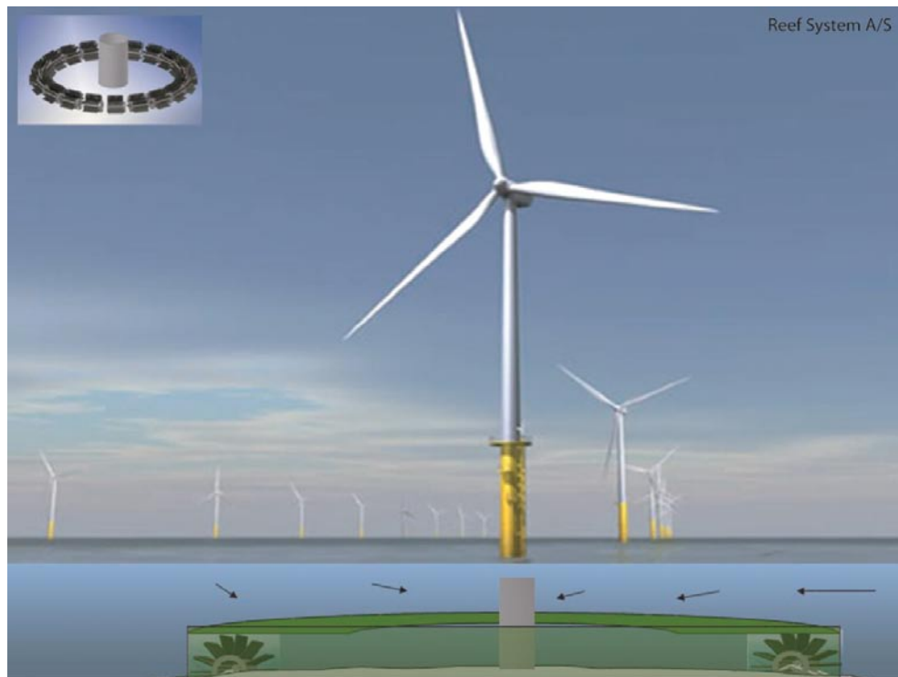
Figure 8. Artificial score protection, GRIP, adjusted to increase the amount of habitat for fish and bottom living animals associated to hard bottom substrate –by the reef-effect. Each module consists of a perforated concrete pipe lined with protruding plastic pipes.
