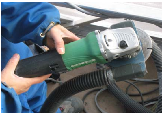
Grinder with metal attachment for dust collection
