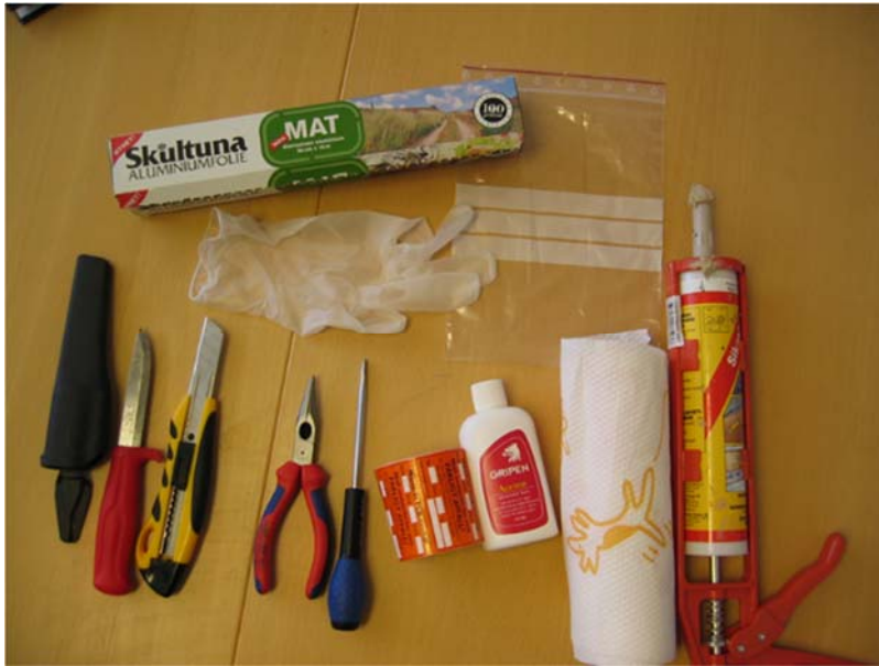
Example of equipment needed for taking samples of sealants
