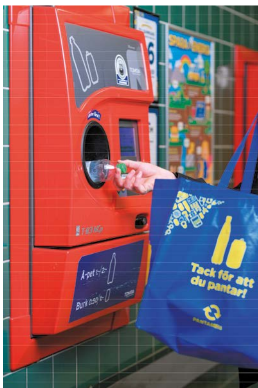
Figure 3. Return vending machine for ready-to-drink bottles and cans at a grocery store. Photo: Returpack/Pantamera.
